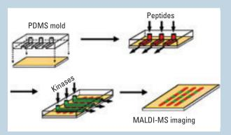
A schematic of a microfluidic peptide array.
